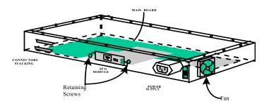
On the rear side of the hub there are two retaining screws for the Bonus Port slot. These are used to secure an SPM module in position. Remove them.
